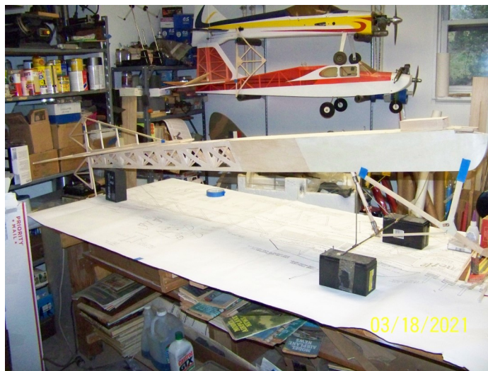
Squaring up the gear assembly
