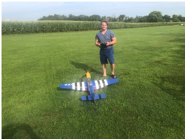
Tim West and his E-flite P-51 1.5m fighter with a SMART 100amp ECS, 6S 50c LIPO, and Power 60 motor, this plane really tears up the skies!
