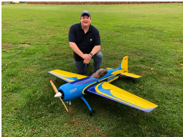
Andy Myers and his Hanger 9 Inverza 33 , this plane utilizes a DLE 35RA gas engine, Spektrum AR12310T 12 channel Powersafe Rx, Hitec 5645 Digital MG Servos, Xoar 19x8 Laminated Prop, and oversized Dubro Tires. I love this plane and have learned so much from it. Interesting fact — The plane was purchased from Jim Christensen who purchased and built the plane new.
