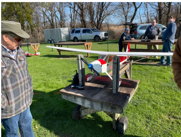
Jim Christensen and his Sig 110" Rascal. This plane sports a DLE 20RA gas engine and Hitec servos. Jim was having problems steering, but that was quickly remedied by adding a custom spring setup to the tail wheel and rudder. This is a lotta plane!
